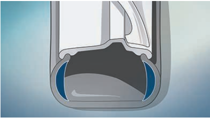
■ Tyre pressure monitor. Sensors on each wheel assess the tyre pressure and temperature and the tyre pressure monitor warns the driver of any loss of pressure.
